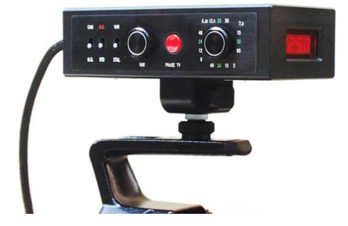
**MULTIQUARTZ** is an highly sophisticated, compact, very low current consumption, electronic device that has been designed and optimised for ARRI 16 SR cameras, factory engineered to work without any modification either with Standard or with High Speed model.
